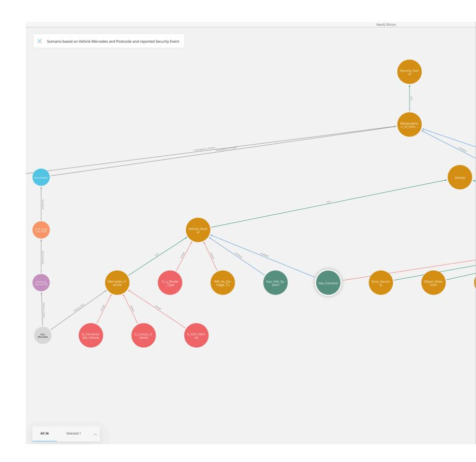
The Vehicle Digital Twin model breaks down into vehicle functions such as Acceleration, Object Detection and Navigation. A domain predicate - Has Failed Service - links to known vulnerability or service history and a range predicate - Has Policy - that refers to Vehicle policy controls such as Security that would detail rules or thresholds.
